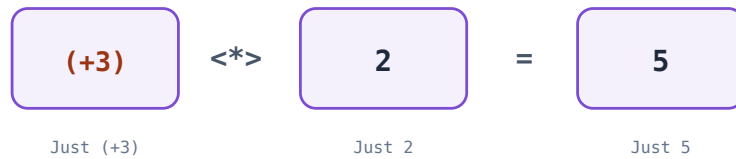
Fig. 2.5. Applicative application: both the function and the value are in a context; ( < * > ) applies the former to the latter and returns the result in the same context.
