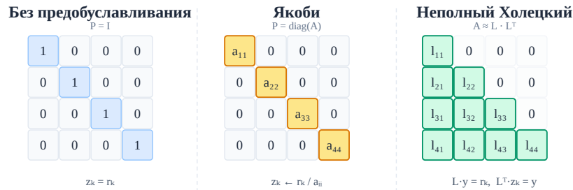
Fig. 3.3. Preconditioners: identity ( P = I ), Jacobi ( P = \text{diag}(A) ) and incomplete Cholesky ( A \approx L \cdot L^T ).
